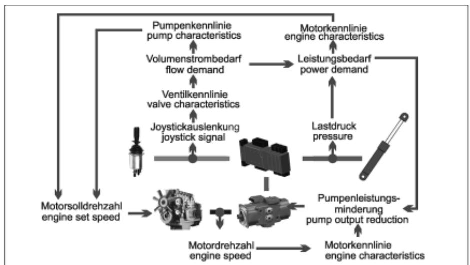
Fig. 1: Information flow in powertrain management of excavators
