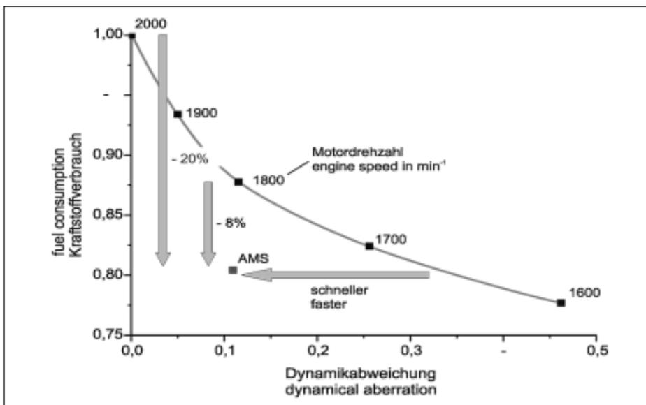
Fig. 2: Fuel consumption and dynamical aberration at partial load
