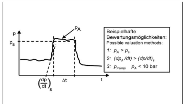
Fig. 2: Electronically controlled Kick Out with different valuation methods
