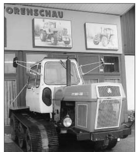
Fig. 3: The ZT 300 tractor as crawler
