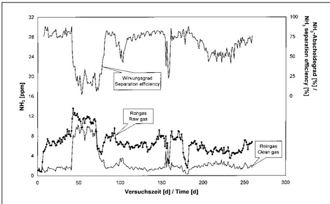
Fig. 2: Time dependent course of ammonia input and output concentrations as well as separating efficiency during cleaning of waste air from piggeries with a two-stage scrubber operating with water
