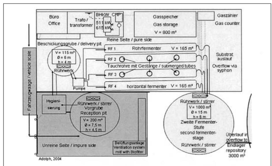
Fig.1: Scheme of the pilot-biogas plant with four horizontal cylindrical fermenters (each  $165 \text{ m}^3$ ), one second stage fermenter (vertical cylinder with  $1000 \text{ m}^3$ ) and gasmotor ( $511 \text{ kW}_e$ ,  $615 \text{ kW}_h$ ) cogeneration unit
