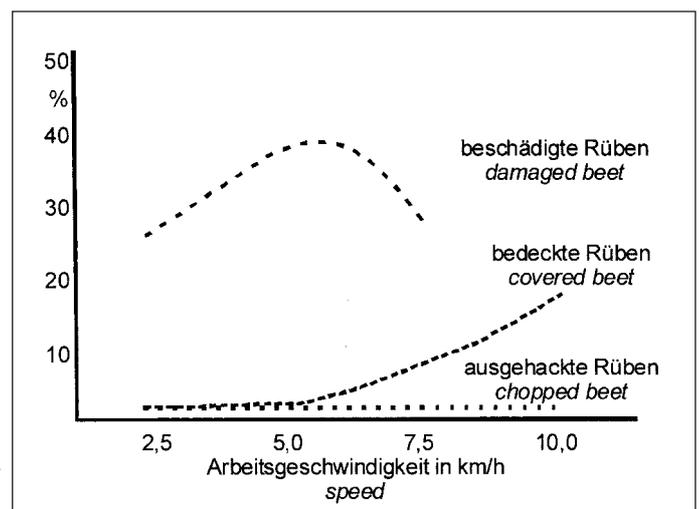
Fig. 1: Effect of driving speed on work quality of hoes ([2] modified)
