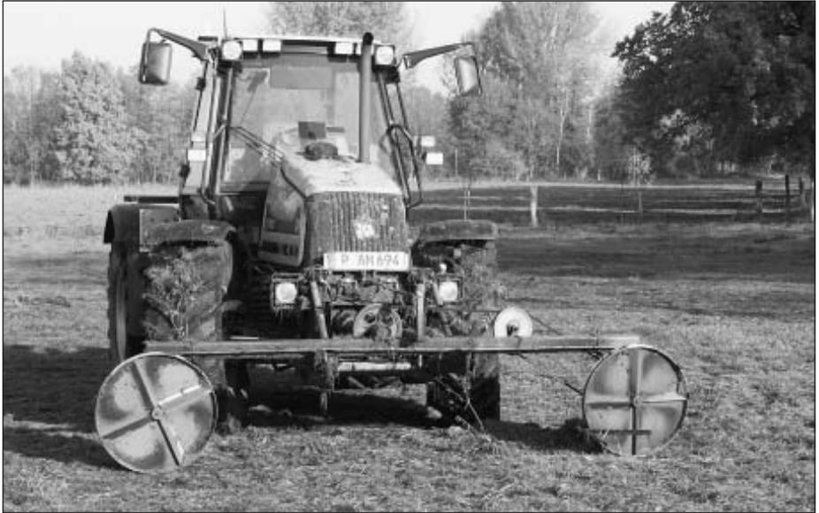
Fig. 2: Second research model of the band mower, 2003
