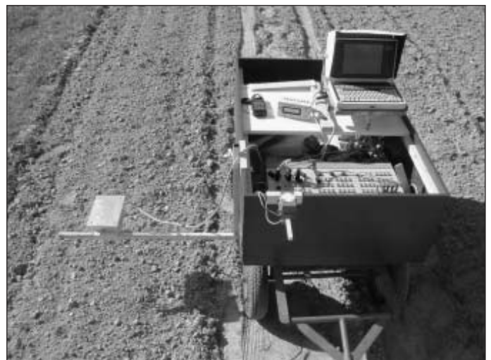
Fig. 1: Field wagon to measure reflection of crops and weeds
