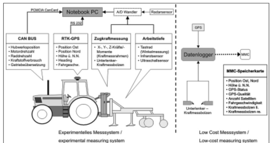
Fig. 1.: Simultaneously used measurement systems for draught force mapping
