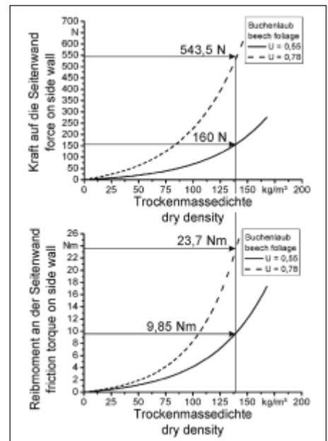
Fig. 3: Force und friction torque on the side wall of the press chamber
