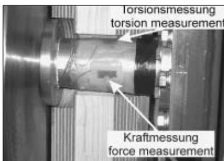
Fig. 2: Sensor for measuring side wall friction
