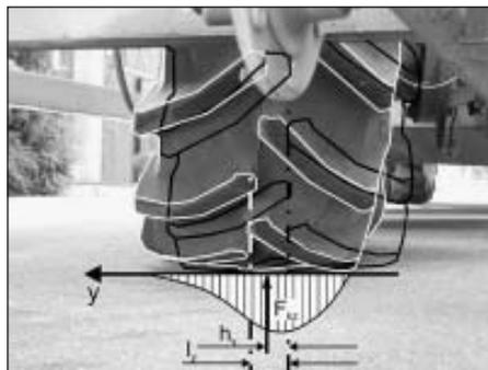
Fig. 3: Picture of a tractor tyre deformed by lateral force with qualitative distribution of pressure displayed. The black contour denotes an unstressed state.
