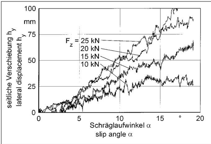
Fig. 2: Lateral displacing of  $h_y$  as a function of the slip angle for different tyre loads. (tyre: 520/70 R34,  $p_i = 0,8$  bar,  $v = 5$  kph, asphalt)
