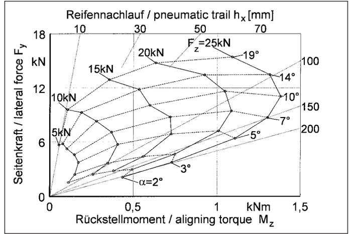
Fig. 4: Relations of lateral force, aligning torque, tyre trail, tyre load and slip angle in the Gough diagram (tyre: 520/70 R34,  $p_i = 0.8$  bar,  $v = 5$  kph, asphalt)
