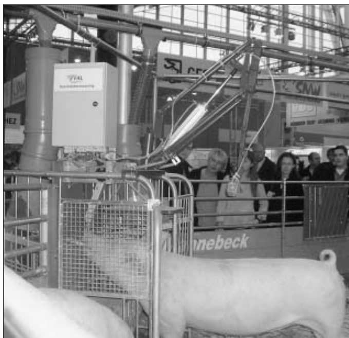
Fig. 1: Automatic backfat-thickness measurement
