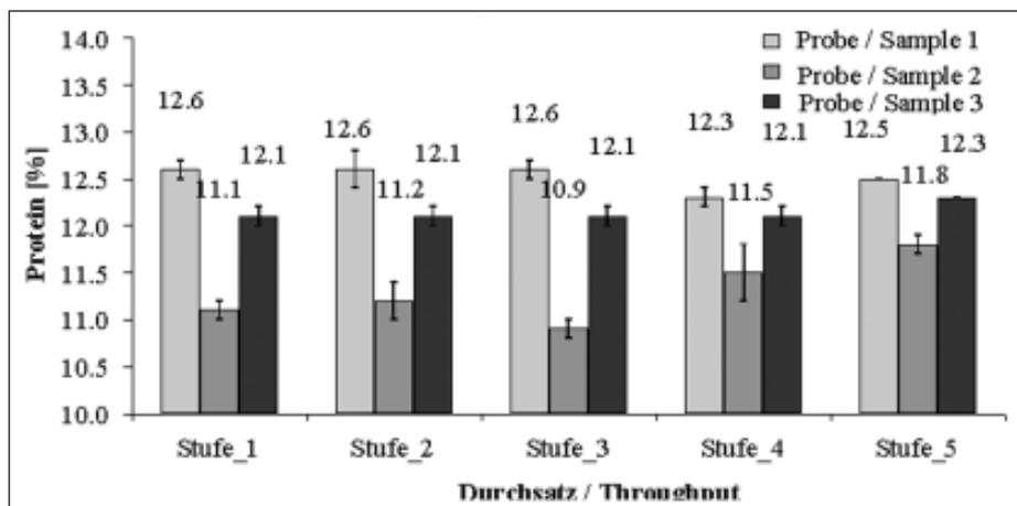
Fig. 3: Influence of throughput on measuring protein (calibration 2)
