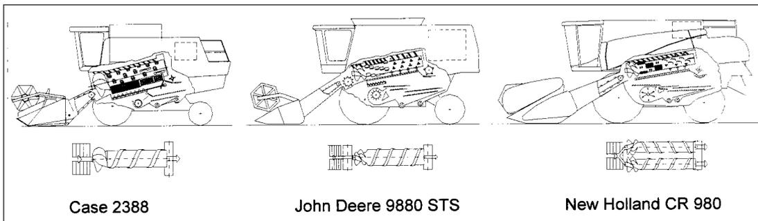
Fig. 3: Cross section and material flow of rotary combines, offered in Germany
