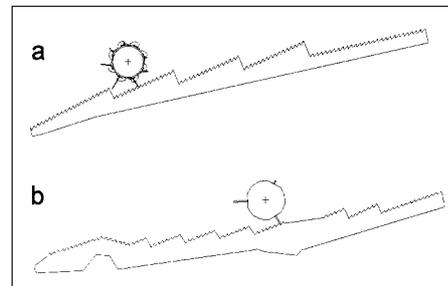
Fig. 2: Rotary elements for grain separation improvement
