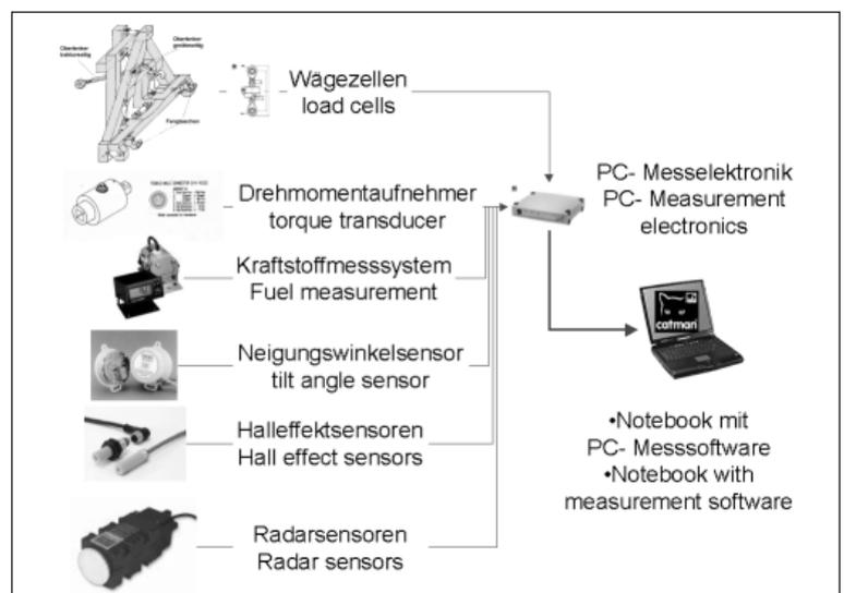
Fig. 1: Measuring technology used during experiments
