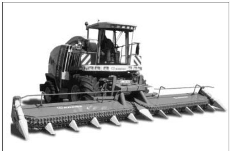
Fig. 3: Self-propelled forage harvester Big X (Photo Krone)
