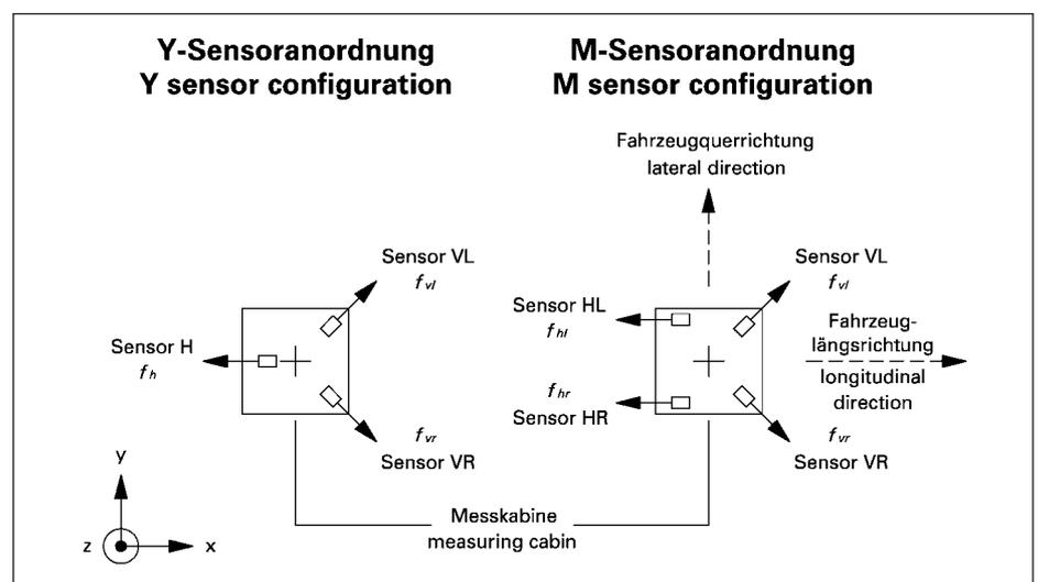
Fig. 1: Position of sensors
