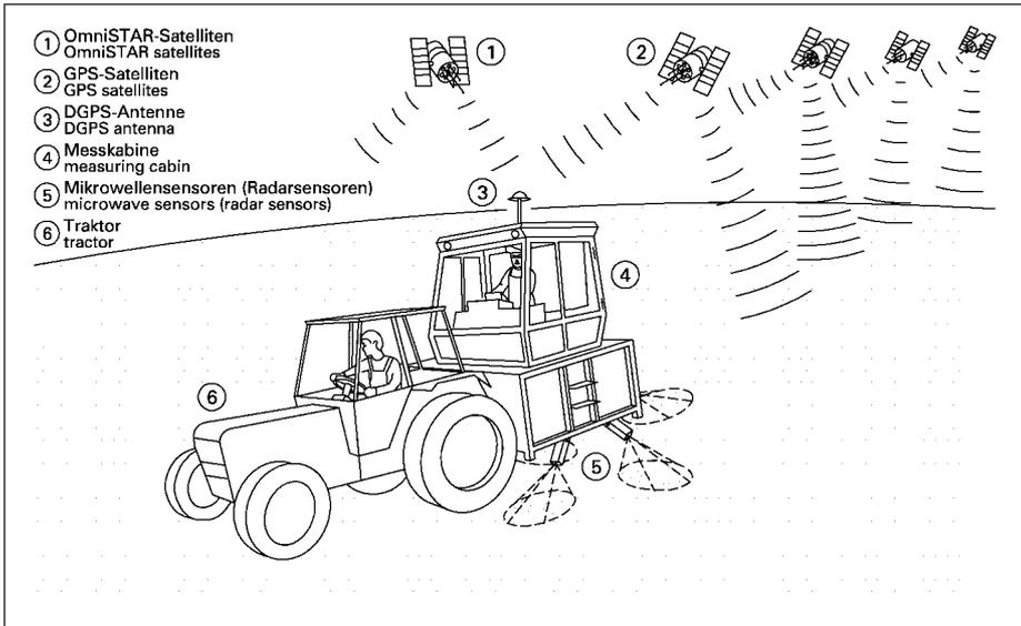
Fig. 2: Field measurement setup
