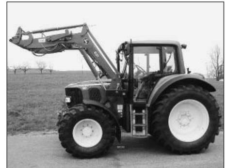
Fig. 1: Tractor with front loader
