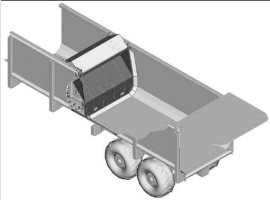
Fig. 1: Transport wagon with moveable push-blade
