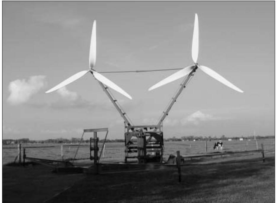
Fig. 2: Erected mobile wind energy plant MoWEC
