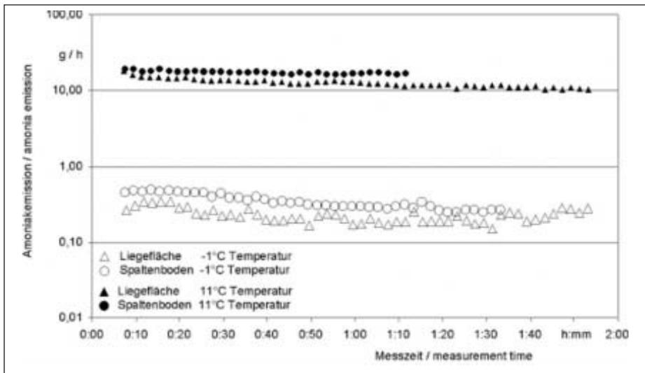
Fig. 1:  $\text{NH}_3$ -emissions above pig house floors with different fresh air temperatures measured by a wind tunnel
