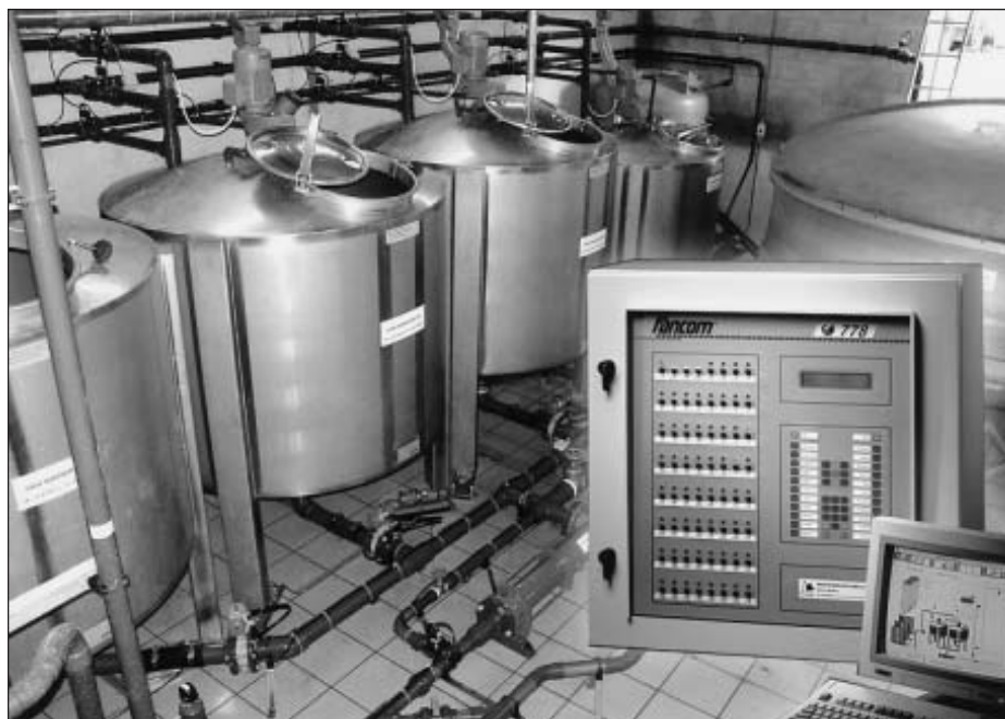
Fig. 2: The liquid feeder computer 778 by Fancom controls automatically complex mixing rooms of large farms
