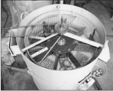
Fig. 2: Prototype of the mechanical peeler.
