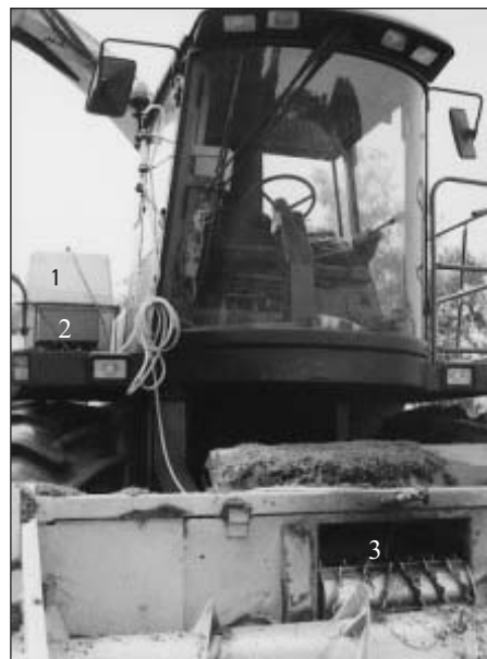
Fig. 3: Forage harvester with device for spraying the harvested grass with starter culture suspension; 1 storage tank for starter culture suspension, 2 dosage pump, 3 spray nozzle
