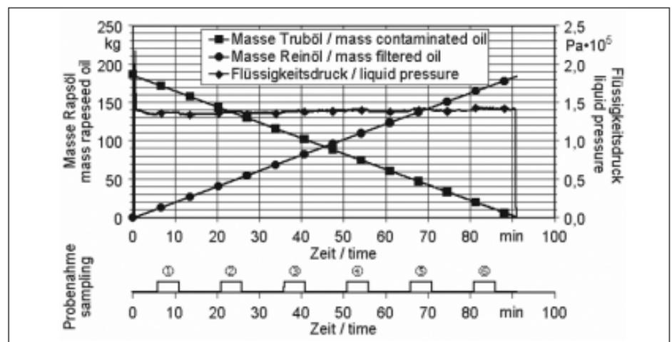
Fig. 1: Alteration of mass and liquid pressure as well as sampling during the filtration of rape oil with a cotton-candle filter
