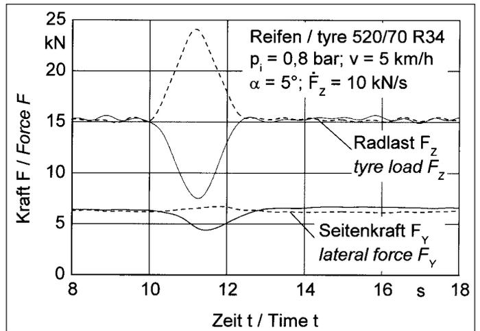
Fig. 3: The progression of wheel load and lateral force during ramp induced wheel load change
