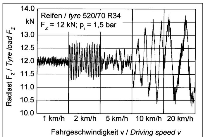
Table 1: Wheel load shock factors for differing road surfaces:  $F_z$  static wheel load,  $P_i$  inflation pressure,  $v$  driving speed,  $S_e$  shock factor loading,  $S_b$  shock factor unloading
