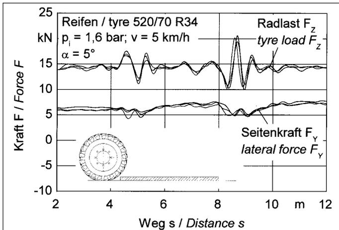
Fig. 2: Course of wheel load and lateral forces driving over a step with three repetitions
