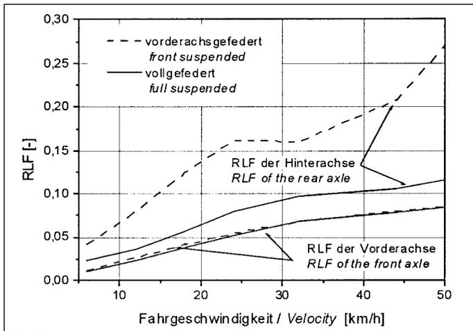
Fig. 1: Comparison of wheel load factors at front and rear axle of an unloaded vehicle according to driving speed
