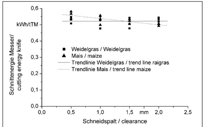
Fig. 4: Cutting energy depending on clearance for raigras and maize (cutting velocity 5 m/s)
