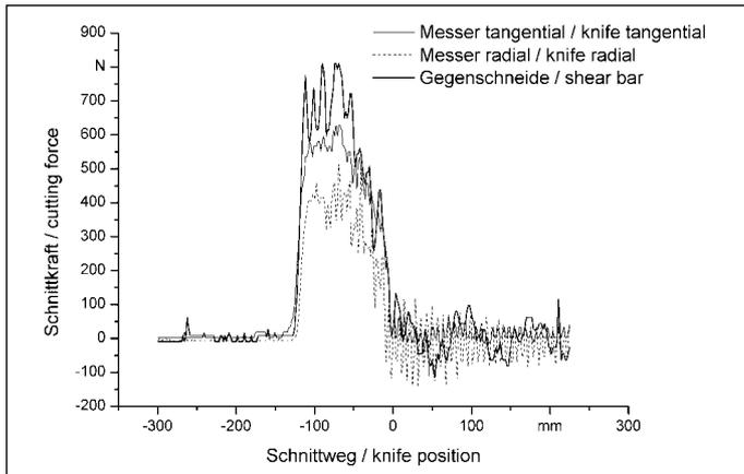
Fig. 3: Cutting forces at cutting velocity of 5 m/s applied to raigras
