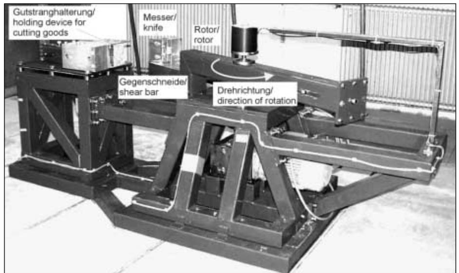
Fig. 1: Cutting test rig
