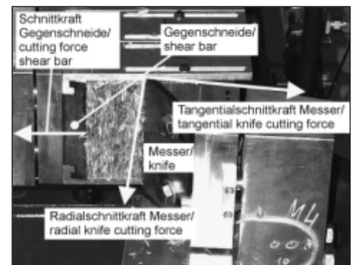
Fig. 2: Force measurement at knife and shear bar
