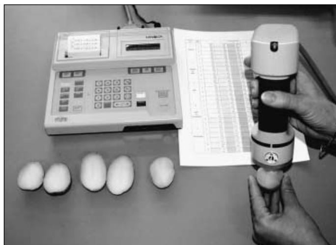
Fig. 2: Determination of potato flesh colour via Minolta ChromaMeter
