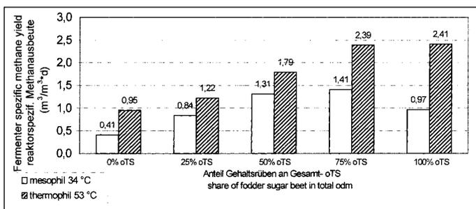
Fig. 3: Fermenter-specific methane yield with mesophilic and thermophilic fermentation (34 °C) of liquid cattle manure and liquid fodder beet silage under 15 days of hydraulic retention time
