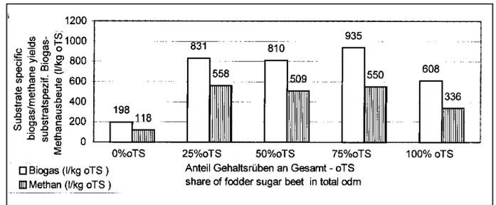
Fig. 2: Substrate-specific biogas/methane yields with mesophilic fermentation (34 °C) with different proportions of liquid fodder beet silage and cattle slurry under 20 days of hydraulic retention time
