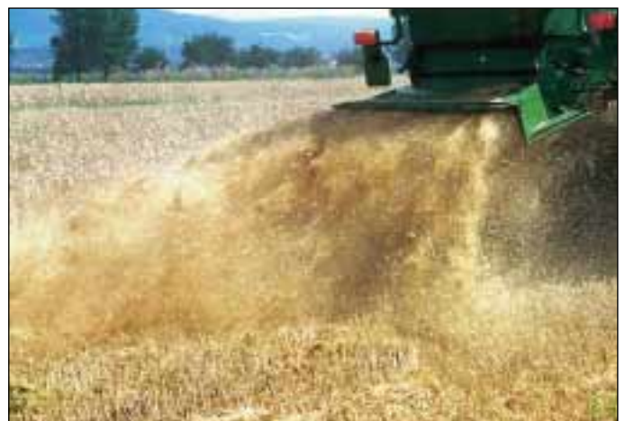
Fig. 1: Visible differences of straw distribution of test chopper with modification on one side
