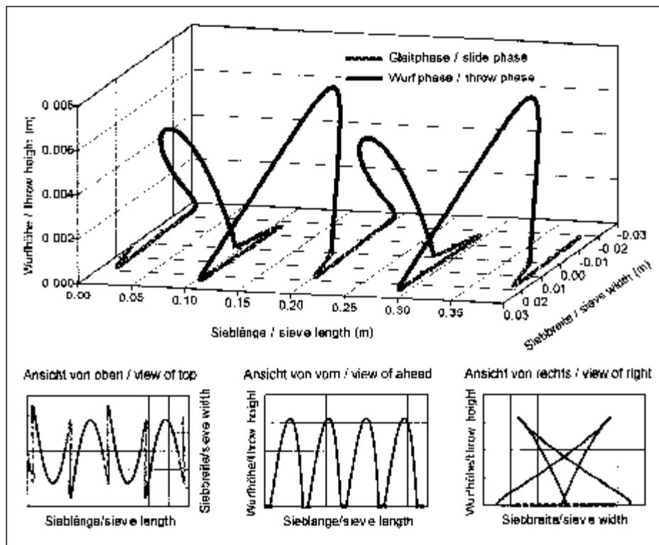
Fig. 2: Motion trajectory relative to sieve with SV = 1.5
