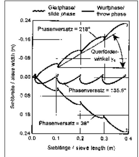
Fig. 4: Motion trajectories relative to sieve by  $SV = 1$
