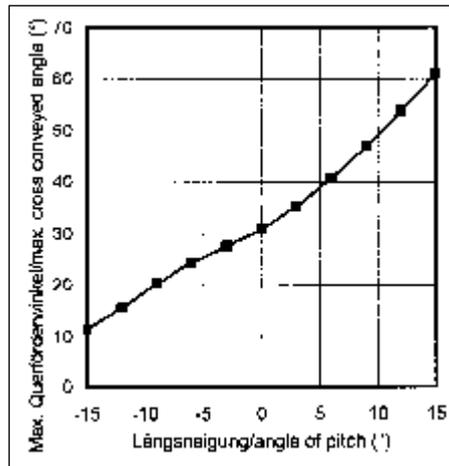
Fig. 7: Angle of pitch influence of max. cross conveying angle
