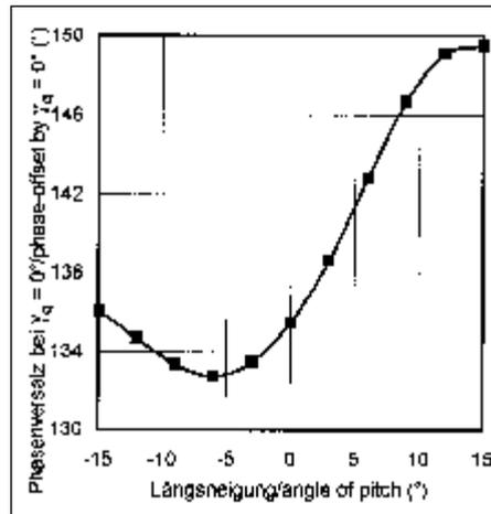
Fig. 8: Angle of pitch influence of phase-offset by cross conveyed angle  $\gamma_q = 0^\circ$
