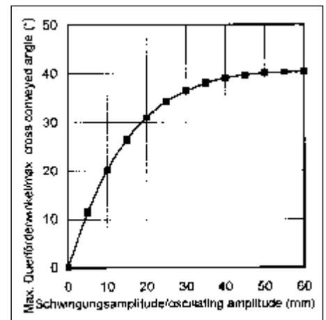
Fig. 6: Influence of oscillating amplitude  $a_z$
