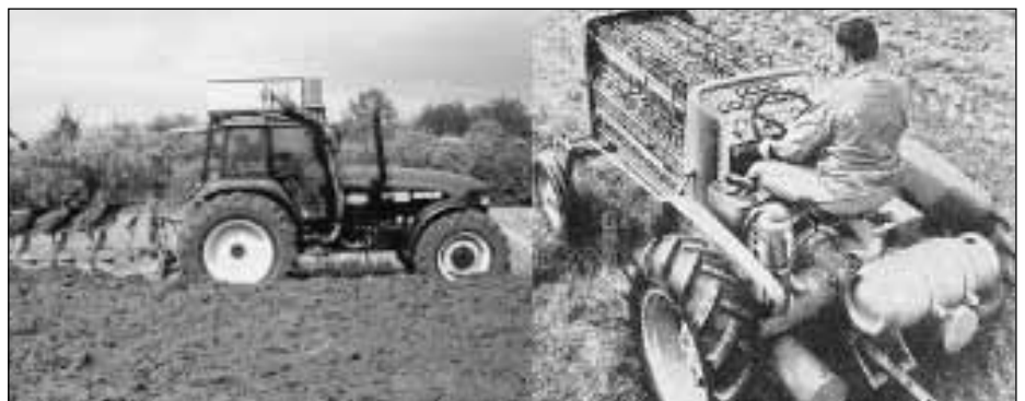
Fig. 1: Diesel-electric tractor by Schmetz and fuel cell tractor by Allis Chalmers
