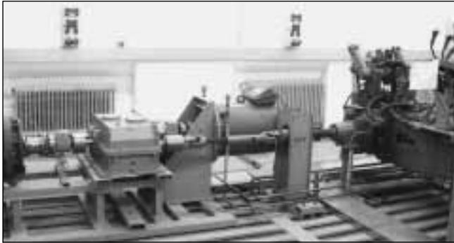
Fig. 13: Transmission test bench of the TU Dresden
