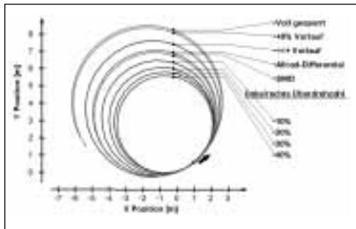
Fig. 14: Trajectories of the geometric tractor center
