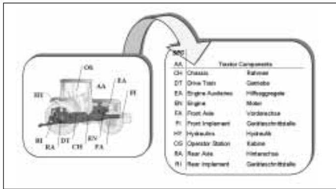
Fig. 7: SFC basic structure of tractors
