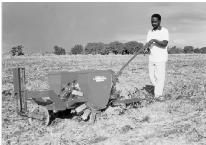
Fig. 3: Animal-Drawn Revolving Spade-Punch Planter (ADSP) in work
