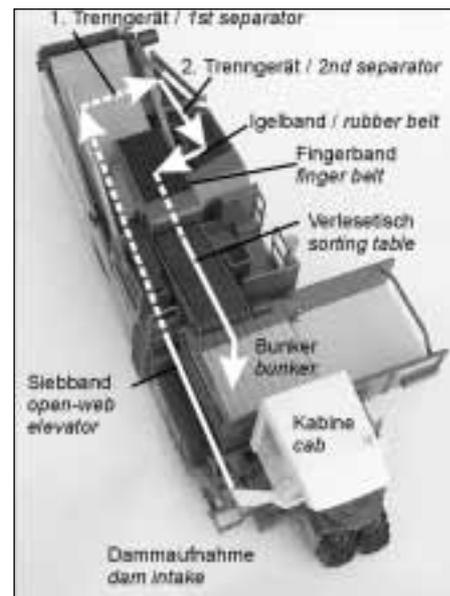
Fig. 1: Potato tracing through the harvester
