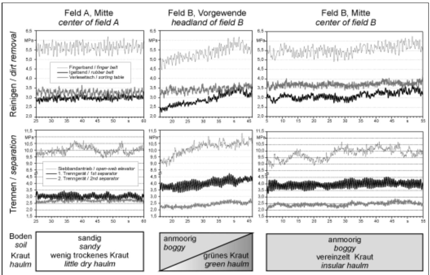
Fig. 2: Pressure readings from separation and dirt removing devices at different operating conditions
