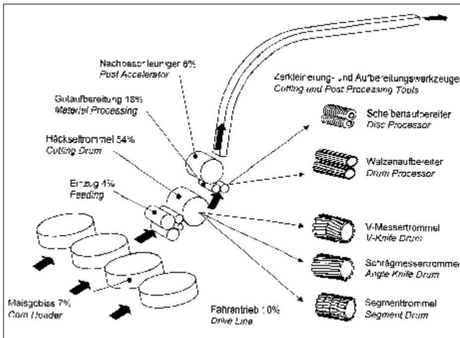
Fig. 2: Chopping process with material flow, design of cutting and post processing tools and power distribution (forage maize)
