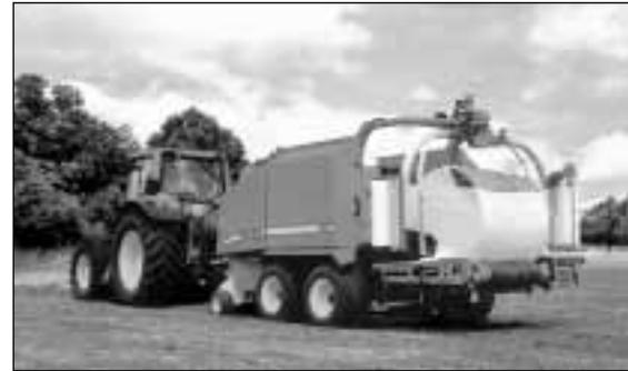
*Fig 3: Wrapping of round and big square bales has developed. A number of exhibitors offer improved labour efficiency through combining baling and wrapping in one machine. Here, the John Deere 678 combination baler which avoids the need for separate wrapping operations in the field.*
