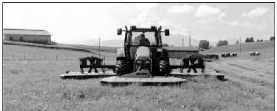
Fig. 1: The mower combination KM5.90 from Deutz-Fahr in „butterfly“ mode (two mowers rear, one front-mounted) gives a working width of 8.50 m.
