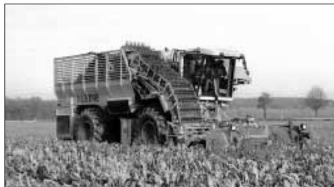
Presented by Kleine at Agritechnica is the low ground pressure SF 2002 sugar beet harvester. This attribute is achieved through lower net weight of 21.3 t with 20 t sugar beet capacity through completely new design and four tyres of 1.10 m breadth.
