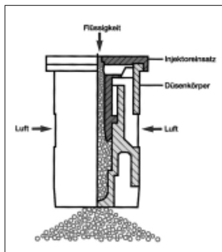
Function diagram of Lechler IDK air injector compact jet
