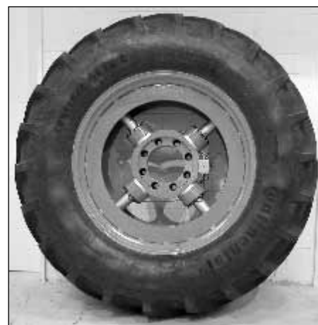
Fig. 1: Instrumented wheel with tire 520/70 R 38
