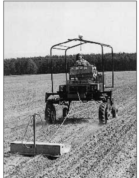
Fig. 1: Equipment for measuring electrical soil conductivity (EM-38)
