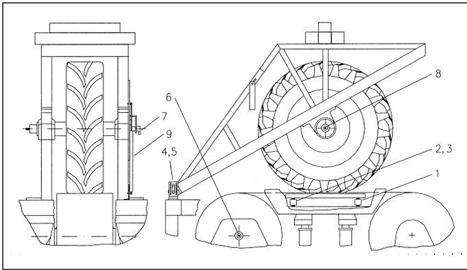
Fig. 1: Flat-belt tyre test stand
