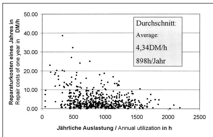
Fig. 1: Repair cost of tractors with different annual utilisation
