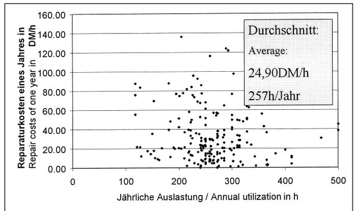
Fig. 3: Repair cost of combines with different annual utilisation
