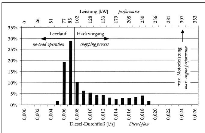
Fig. 2: Extent of utilization of the chopper system with regard to installed power
