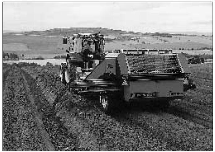
Fig. 2: The separation implement REL 5154S deposits clods and stones via a lateral conveyor belt.
