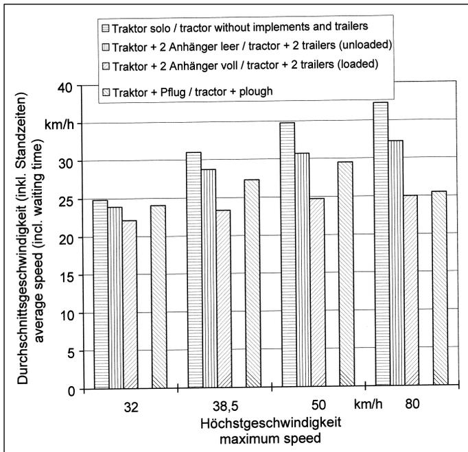
Fig. 1: Average transport (incl. laid-up time), depending on maximum speed determined by design
