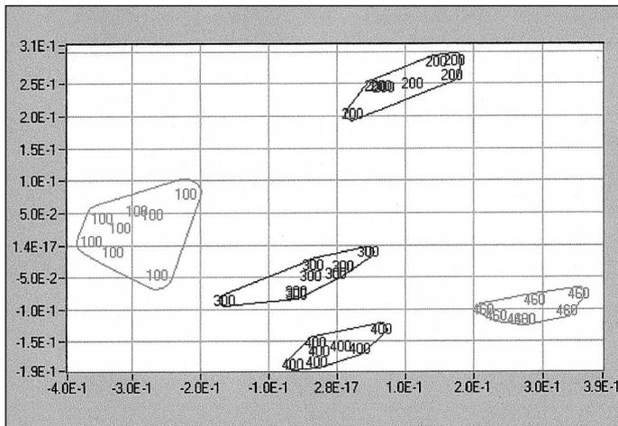
Fig. 1: PCA-plot for different concentrations of n-butanol (100 ppb, 200 ppb, 300 ppb, 400 ppb, 460 ppb)
