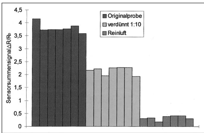
Fig. 2: Results of the MSA measurements from different concentrations of piggery air
