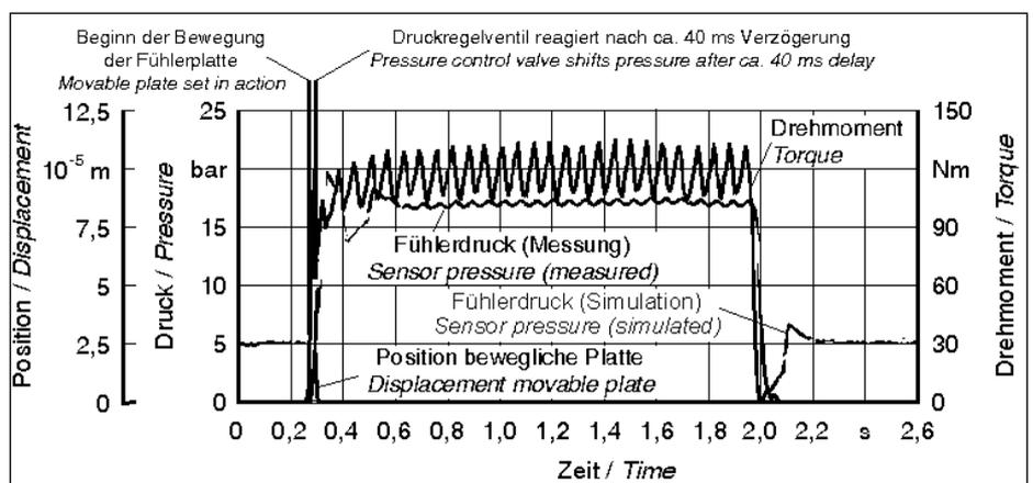
Fig. 4: "Pumping function": compensation for the time delay in the pressure control loop
