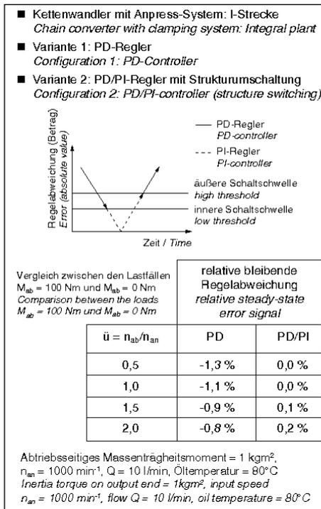
Fig. 2: Suitable structure of ratio control minimises load-dependant steady-state error
