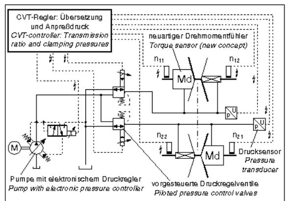
Fig. 3: New concept for CVT hydraulic with pressure control
