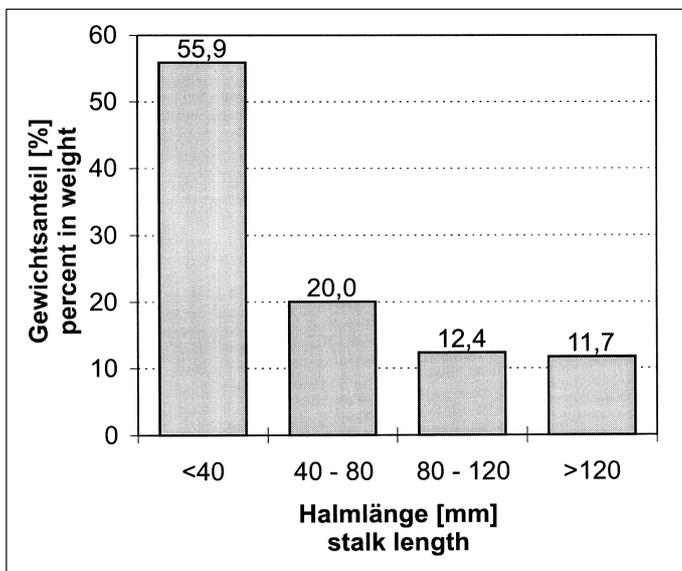
Fig. 2: Straw length distribution in a chopped straw sample (winter wheat, moisture content 32%, throughput 5 kg/s, 4200 rpm)
