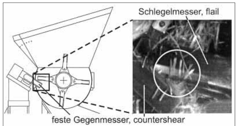
Fig. 3: High speed recording of the chopping procedure at 3200 rpm
