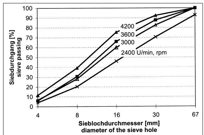
*Fig. 1: Sieve analyses of chopped straw samples at various rpm (material moisture 32%, throughput 5 kg/s)*
